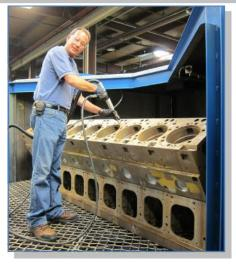
After cleaning, technician used the StingRay Vacuum Gun to remove solution from blind holes and return the solution to the wash machine reservoir.
