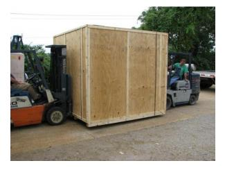
Forklifts are a good choice to move or lift a machine. Be sure the forks extend and pick the load from the machine perimeter base. Do NOT lift on the machine floor.
