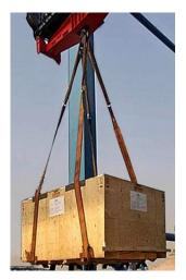
Single point lifting is never the first recommendation nor should you choose this method if other better options are available. However, under certain conditions it is possible to lift the crate from a single point without damage. Be sure the lift point is many feet above the crate so the lifting lines are as straight as possible. DO NOT USE short lines with the hook point a couple of feet above the crate.
