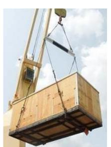
A single spreader beam with sufficiently long straps, chains or cables can be used as the base of the crate can support the transverse lifting loads. Be sure to anchor lift points to the crate to prevent slippage. Using short lifting points
