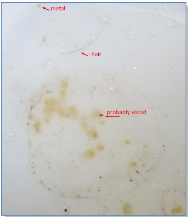
close-up of millipore filter media inside of protective case
