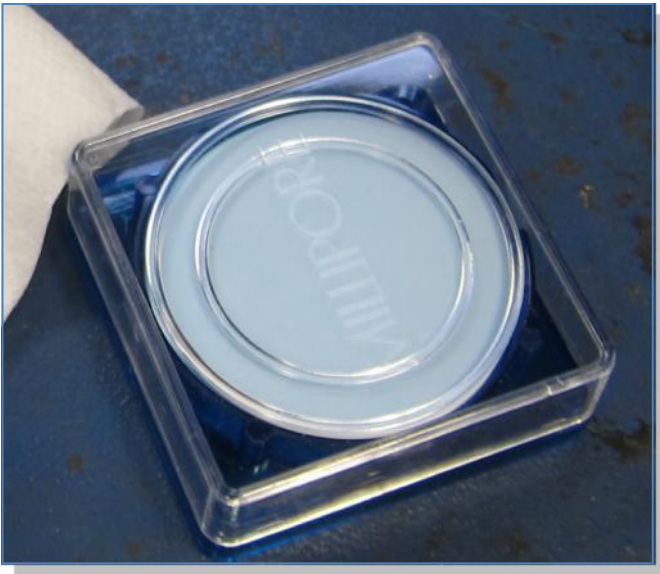
close-up of millipore filter media inside of protective case
