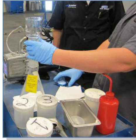
Step Three: Filter collected solvent through Millipore Test Set-Up
