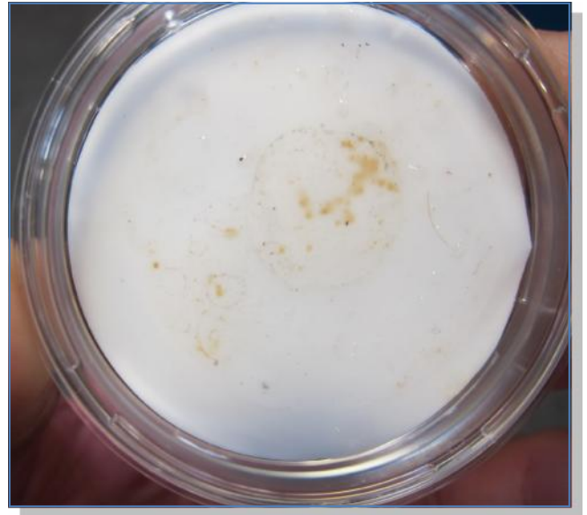
View of filter media after pouring sample through it and vacuumed dry
